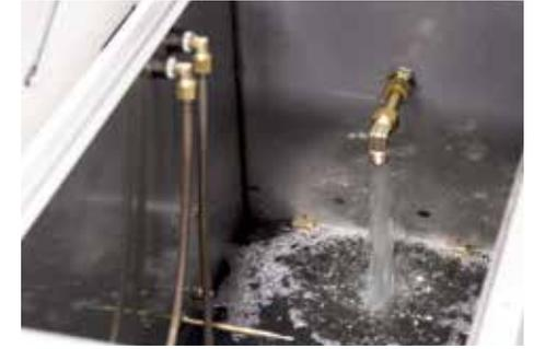
▲ **Dual wash-out tank** for digital flexo plates: Digital wash section for black mask removal is separated from the main solvent tank for easier maintenance and perfect wash-out results.
